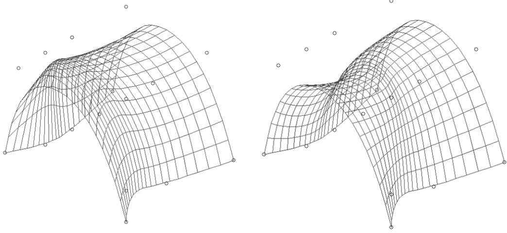
Figure 2: The influence of the weights on the shape of the NURBS surface,  $w_i = 4.0$ ,  $w_i = 0.2$ , (FemDev)
