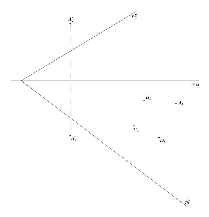
Construct a section of an oblique pyramid ABCDV through a plane  $\rho$ . The base ABCD of the pyramid lies in the horizontal projection plane, a point V is the apex of the pyramid.
