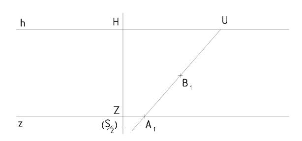
Ex. PP(h, H, z, d/4): construct perspective projection of cube with one wall  $ABCD \subset \pi$ . The tipped ground plan of this wall is given.
