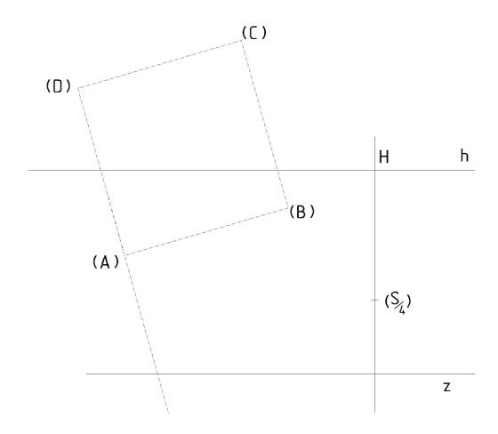
Ex. Find tipped ground plan of  $\Delta$  *ABC*  $\subset \pi$ , its perspective projection is given.
