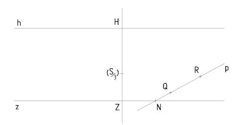
Ex. PP(h, H, z, d/2): construct perspective projection of cube  $A_1B_1C_1D_1ABCD, A_1B_1C_1D_1$  in  $\pi$ ,  $A_1 \in z$ .
