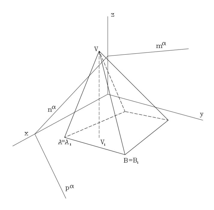
Construct the plane section of the skewed prism by the plane  $\alpha$ . The base of the solid is in the horizontal plane.
