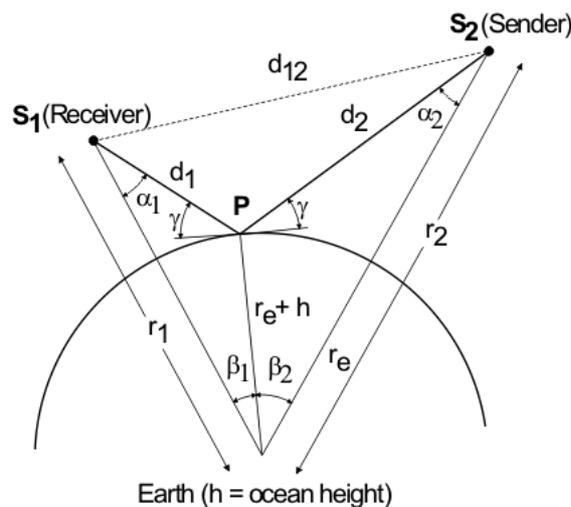
Fig. 1: Principle of bistatic altimetry [3]
